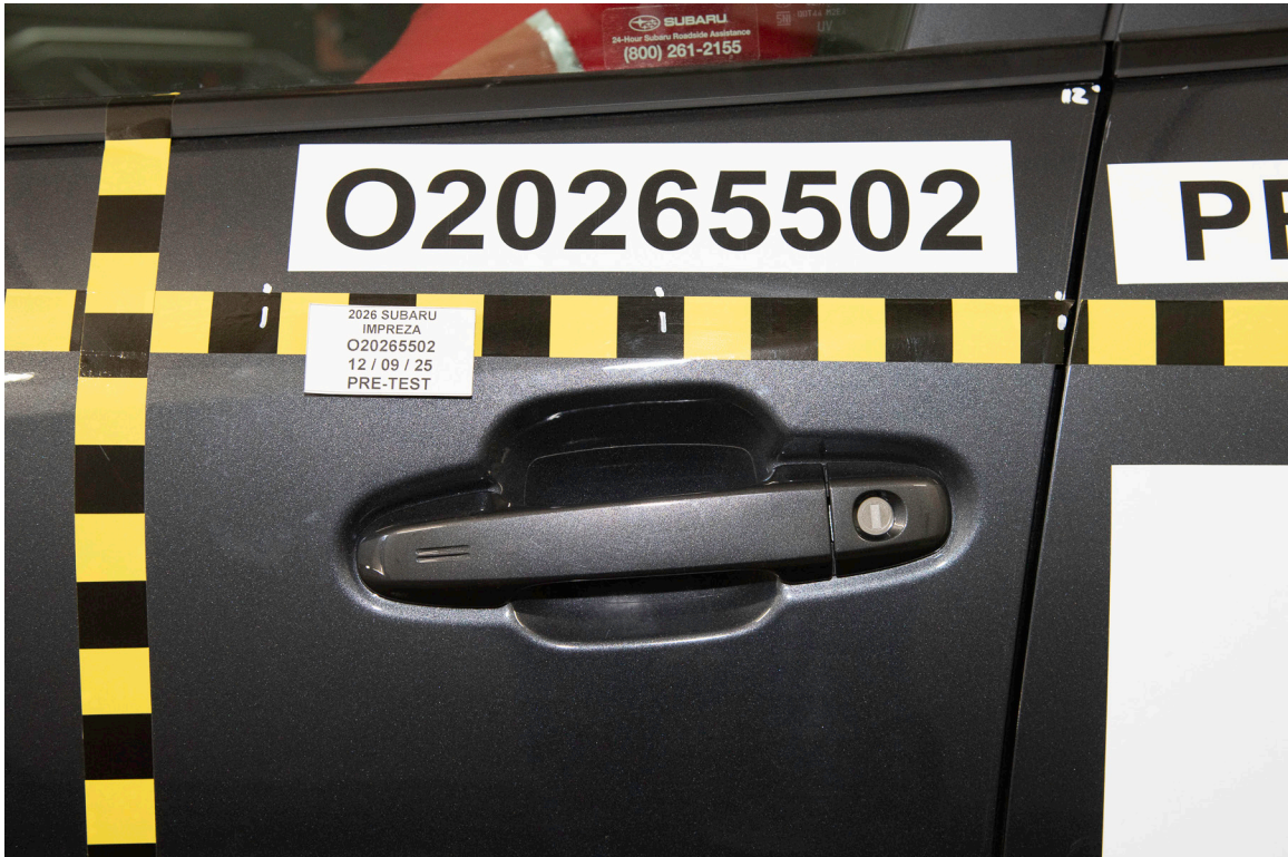
FIGURE 21. Pre-Test Left Front Door Latch Close-Up
